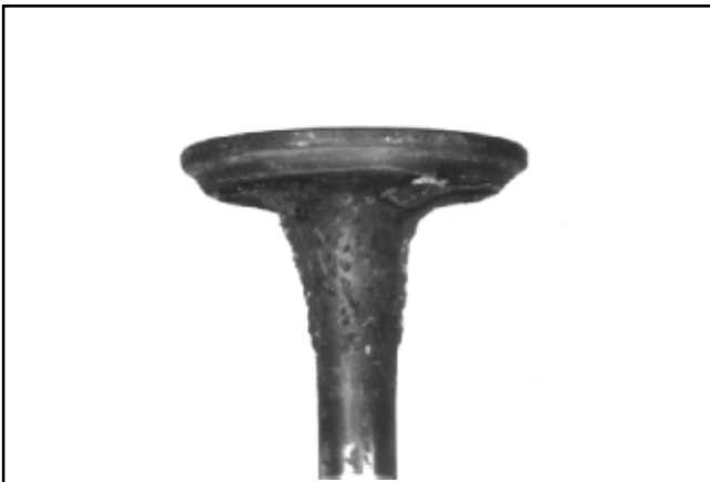
Gum: Gum deposits usually result from using stale gasoline. Gum is a prevalent cause of valve sticking. The cure is to ream the valve guides and clean or replace the valves, depending on their condition.
